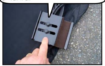
STEP 3: WITH THE REAR BRACKETS EXTENDED THEY WILL SIT ON TOP OF THE SIDE OF THE REAR TRIM PANEL.
