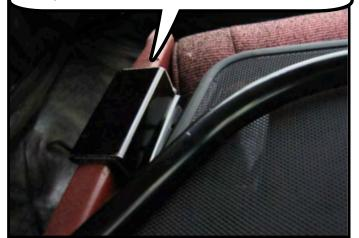
STEP 4: FROM UNDERNEATH THE WIND DEFLECTOR PULL BACK ON THE REAR BRACKET AND THEN TIGHTENED THE THUMB SCREWS HOLD THE WIND DEFLECTOR IN PLACE. REPEAT ON THE OTHER SIDE.
