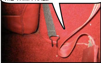
THE STRAPS WILL ATTACH TO THE BUCKELES ON THE BOTTOM OF THE WIND DEFLECTOR.
