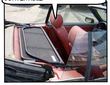
THE WIND DEFLECTOR ATTACHES TO YOUR MUSTANG WITH TWO FRONT BRACKETS AND TWO REAR BRACKETS. THE REAR BRACKET IS ADJUSTABLE AND LOCKS THE WIND DEFLECTOR IN PLACE.
